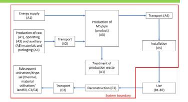
The following is a detailed list of the life cycle stages and process modules taken into account in the manufacture of the pipe:
